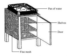
Figure 6 Evaporative cooler with rice husk as cooling pad
