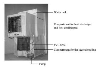
Figure 11 Indirect active evaporative cooler
