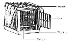
Figure 5 Evaporative cooler with jute bag as cooling pad
