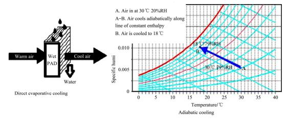
Figure 1 Schematic of direct evaporative cooling (Source: www.ecocooling.co.uk/psychr.html)
