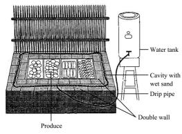
Figure 7 Evaporative cooler made from bricks
