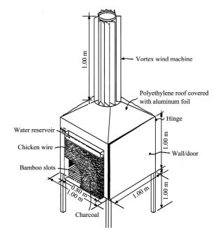
Figure 9 Evaporative cooler with vortex wind machine
