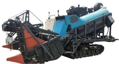
Figure 1 Overall structure of rape combine harvester
