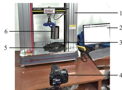
1. HY-0580 universal material tensile and compression testing machine
