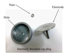
Figure 1 Electrodes of ohmic heater
