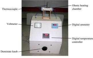
Figure 3 Experimental setup
