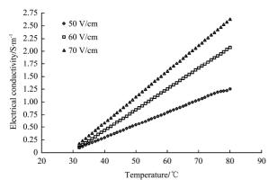
Figure 4 Electrical conductivity of tomato juice during ohmic heating at different voltage gradients
